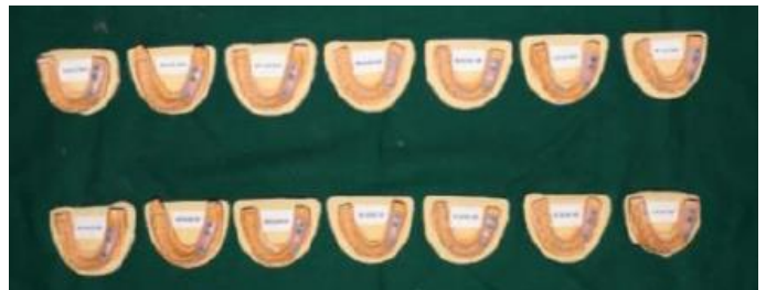
Figure 9: 14 models were with type 4 dental stones from non-splinted impressions
